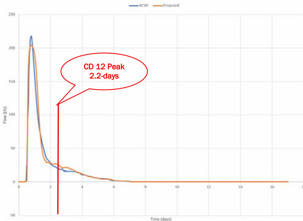
Figure 4. CD 20 Outlet 5-Year Peak Flow Hydrograph Comparison
